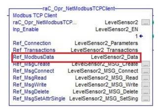
This tag contains four separate data areas for coils (0xxxx), discrete inputs (1xxxx), input registers (3xxxx) and holding registers (4xxxx). These tag values can be read and populated by the user application without any restrictions.
