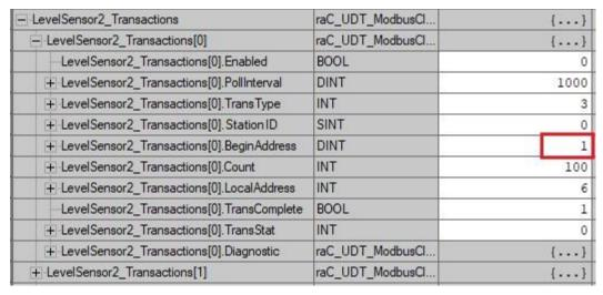
6. Set **Count** tag. The value represents the number of items in remote device (Modbus TCP Server) to read from or write to.
