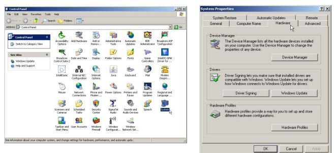
Navigate to the item Ports (COM & LPT), and select the Prolific USB-to-Serial Comm Port cable from the list. If the assigned port is COM1, COM2, COM3 or COM4, there are no other steps required. Simply make note of the assigned COM port number.
