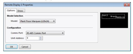
3. Any items placed 'inside' of the Remote Display box will be displayed on the attached PFM.
