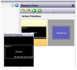
2. Open the Remote Display primitive's properties, set the Model Comms Port and Unit Address appropriately.
